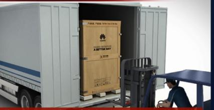
Then, slowly insert the two forks into the clearance to avoid scratching.
